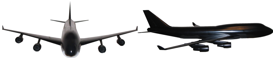
Figure 3-21: The plastic, 1:100 scale model manufactured by HobbyCraft of Canada. It is painted with an ultra flat black primer and a gloss black topcoat.
